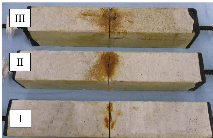
Figure A.23 – Specimens 0.8 mm - #1 after accelerated corrosion test
