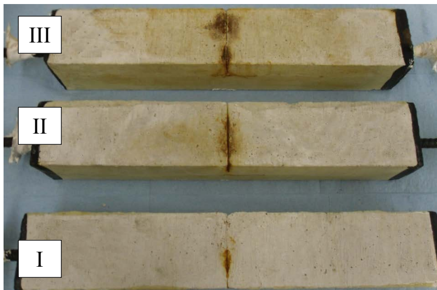
Figure A.20 – Specimens 0.2 mm - #1 after accelerated corrosion test
