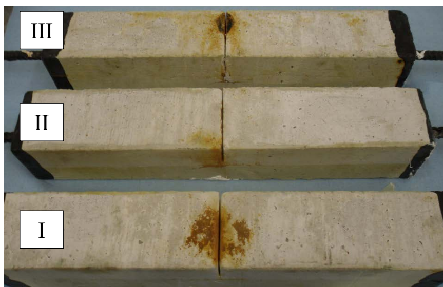
Figure A.25 – Specimens 0.8 mm - #3 after accelerated corrosion test
