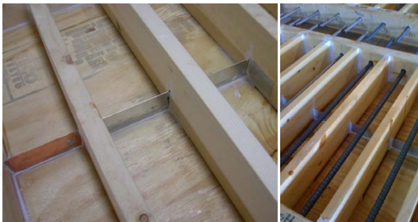
Figure A.19 – Mold detail. Metallic insertion for pre-notch
