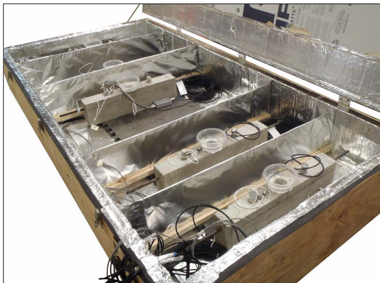
Figure A.28 – Accelerated corrosion test setup
